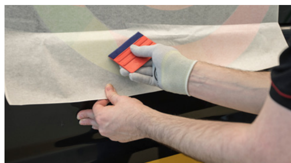
Using Application Paper 300 - High Tack to apply a printed reflective V-4000 signage.
